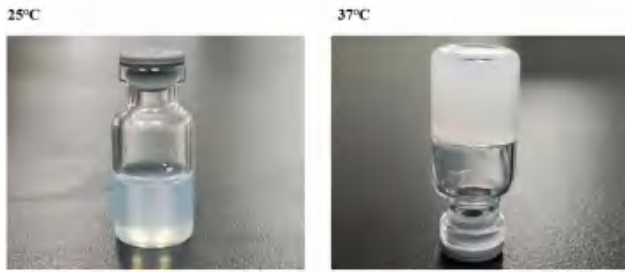
图 1 温敏凝胶的外观性状的优选 Fig 1 Appearance traits of preferred prescription of temperature-sensitive in situ gel
